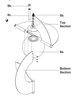
**3.** Attach bottom section to top section with screws **(6a)**, followed by screw cover **(6c)** and secure with finial **(6b)** by threading clockwise
